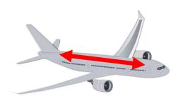
..... of the airplane, is a long hollow tube which holds all the pieces of an airplane together.
